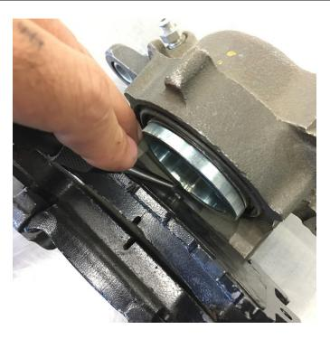
**Kits with non-parking brake calipers** should be checked to confirm the machined pad spacers are present and make sure the notch in the pad spacer lines up with the corresponding boss on the brake pad. If equipped with a pad clip, insert this into the bore.
